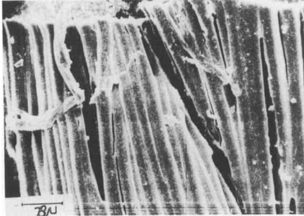
FIGURE 4 Photomicrograph of chopped edge of a twisted Nylon yarn (143×).
